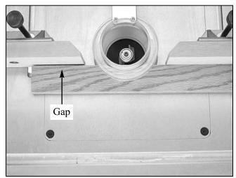
**Figure 17.** Gap indicates amount fence should be adjusted.
